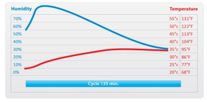
Test with an ambient temperature of 77°F and a humidity of 60%.
