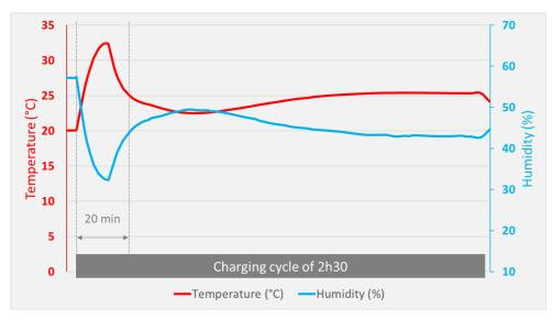
The cycle of the rechargeable PerfectDry Lux starts with a preheating (10 minutes), then is followed temperature by stabilization (10 minutes) in the of the hearing area instruments. This is followed by permanent temperature control around the hearing aids battery for the rest of the cycle time.
